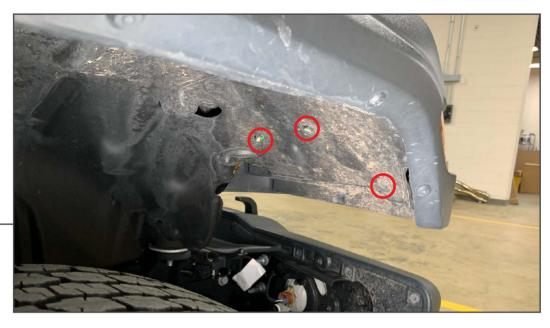
Remove the (2) 8mm bolts and (1) plastic push pin to gain access to the fender mounted running light.
