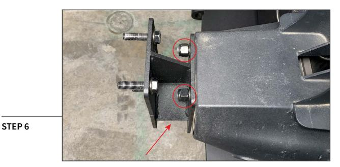
Secure the spare tire relocation bracket to the vehicle tire carrier using (3) 1/2 flat washers and (3) 1/2-20 lock nuts. Tighten all hardware evenly until secure.
