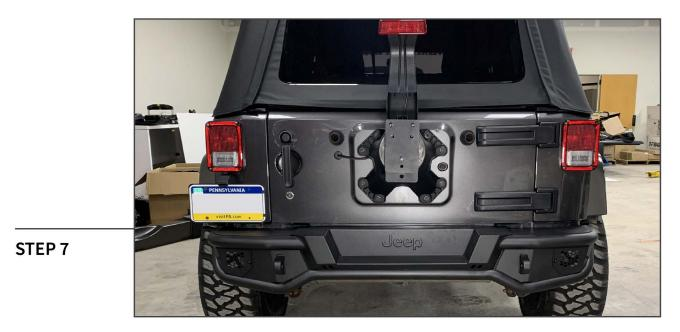
Install the spare tire onto the vehicle tire carrier using the original (3) lug nuts.
