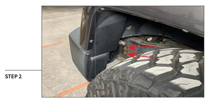
Remove (2) 16mm bolts from each side of the rear bumper. Once removed, pull the bumper away from the vehicle.
