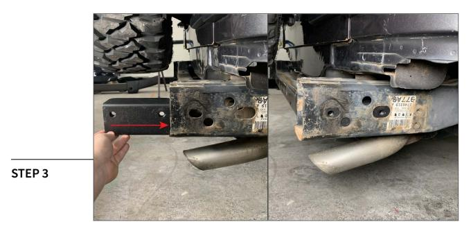
Insert (1) bumper mounting stud plate into the vehicle frame rail, allowing the (2) nuts to show through the pre-drilled holes in the frame.
