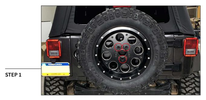
Remove the spare tire from the vehicle by removing the (3) 19mm lug nuts.
