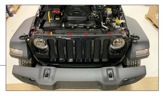
Raise and support the hood to access the (6) push clips securing the grille to the vehicle. Remove the clips and then firmly pull the grille away from the vehicle.
