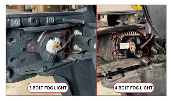
Depending on vehicle trim level, remove the (3) OR (4) 7mm fog light retaining bolts and remove the fog light from the vehicle. Install the new LED fog light with the appropriate mounting adapter to the vehicle bumper reusing the original hardware, and plug in the vehicle wiring harness.
