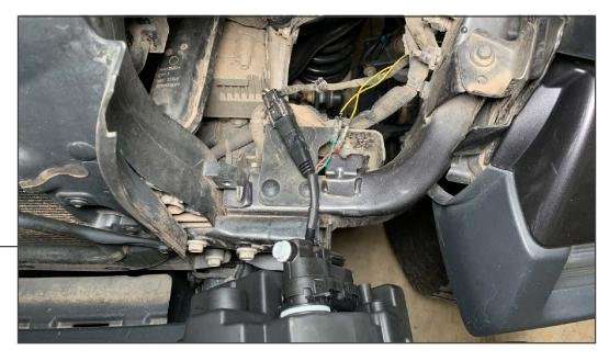
Connect the (2) wire leads to the headlight wiring. Ensure to test functionality before fully connecting the wire leads.
