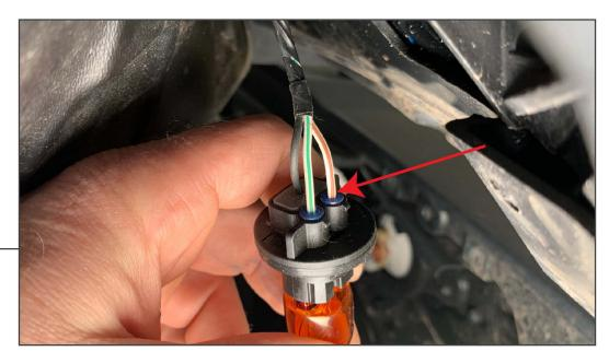
Turn the running light socket counter clock-wise and remove it from the housing. Using a test light, turn on the running lights and test for 12v+ power at the plug. On this vehicle the white/brown wire is the DRL wire. Connect the DRL wire lead (white) to the white/brown wire. Run the spade end of the wire to the headlight bucket.
