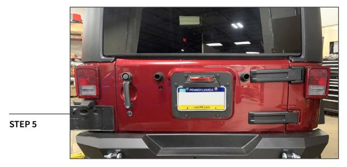
Mount the relocation kit to the vehicle tailgate using the (8) original 13mm bolts. Route the wiring harnesses into the vehicle.
