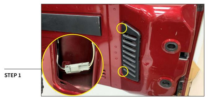
Gently pry along the (2) metal clips to remove the plastic trim cover from the tailgate. Un-plug the third brake light connector from the vehicle.
