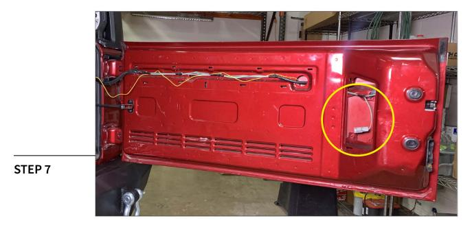
Route the third brake light wiring harness into the vehicle tailgate. Splice the third brake light wiring to the vehicle third brake light harness using the following diagram.
