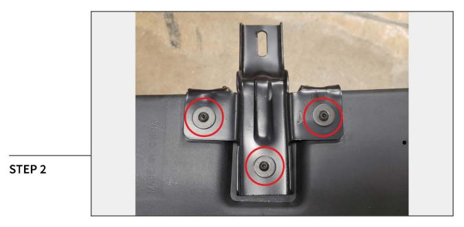
Install the (3) brackets to the side step using (3) M6x1.00 x 20mm bolts and (3) M6 flat washers per bracket.
