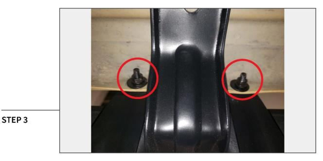
Place the side step into the vehicle pre-drilled pinch weld locations. Secure the side step to the pinch welds using (2) M6 flat washers and (2) M6 nuts per mounting bracket.
