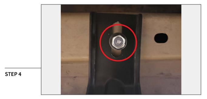
Install (1) M8x1.25 x 20mm bolt and (1) M8 flat washer to secure the upper portion of the mounting bracket to the vehicle body. Fully tighten the (9) M6 bolts securing the side step to the mounting brackets [Step 2].
