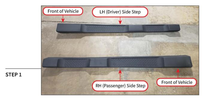
Clean the vehicle pinch weld using exterior detailer and a microfiber cloth. Lay out and identify the side steps. Use the above pictures as a reference.
