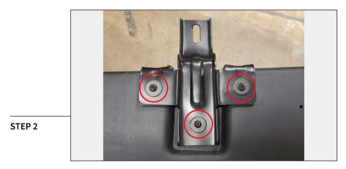
Install the (2) brackets to the side step using (3) M6x1.00 x 20mm bolts and (3) M6 flat washers per bracket.
