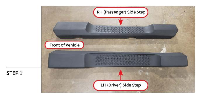
Clean the vehicle pinch weld using exterior detailer and a microfiber cloth. Lay out and identify the side steps. Use the above pictures as a reference.
