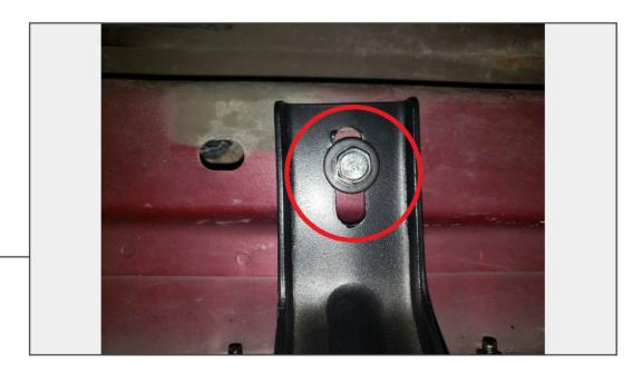
Install (1) M8x1.25 x 20mm bolt and (1) M8 flat washer to secure the upper portion of the mounting bracket to the vehicle body. Fully tighten the (6) M6 bolts securing the side step to the mounting brackets [Step 2].
