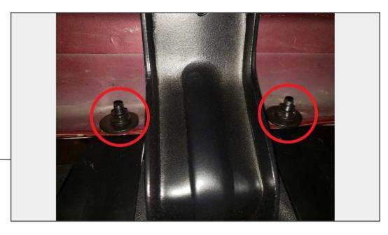
Place the side step into the vehicle pre-drilled pinch weld locations. Secure the side step to the pinch welds using (2) M6 flat washers and (2) M6 nuts per mounting bracket.
