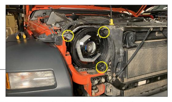
Mount the headlight assembly to the vehicle using the (3) original 10mm bolts. Tighten until secure.
