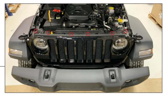
Raise and support the hood to access the (6) plastic push clips securing the grille to the vehicle. Remove the clips and then firmly pull the grille away from the vehicle.
