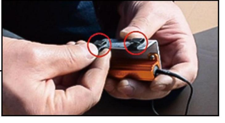
And the black buckle is in the corresponding position of the gasket.
