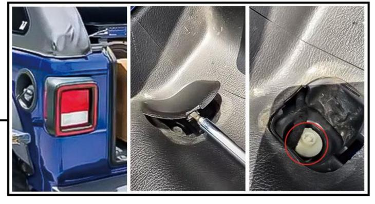
Open the trunk of the jeep, lift a bolt behind the tail light, and remove the white plastic screw.
