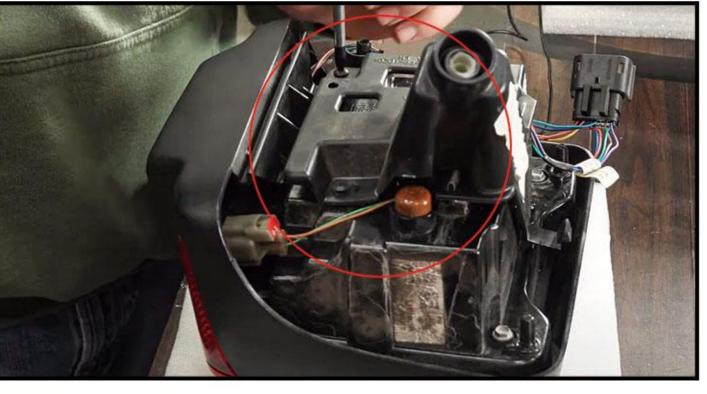
Remove the bracket from the original taillight.
