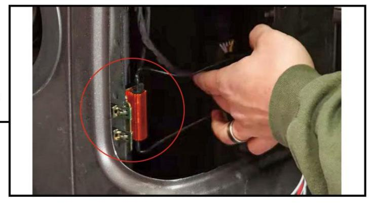
Fix the assembled gasket in the corresponding position of the vehicle.
