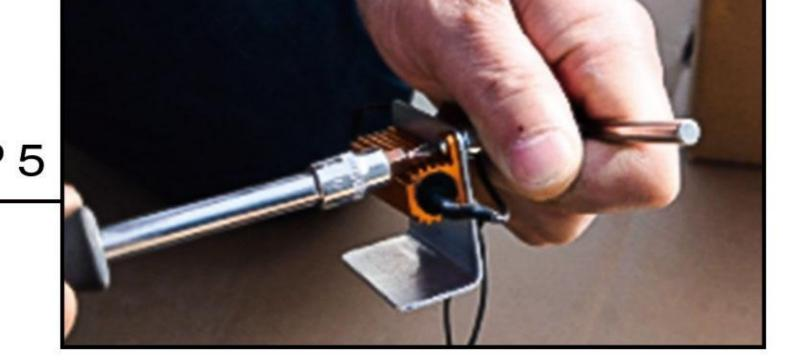
Fix the iron sheet and the resistive decoder with screws.
