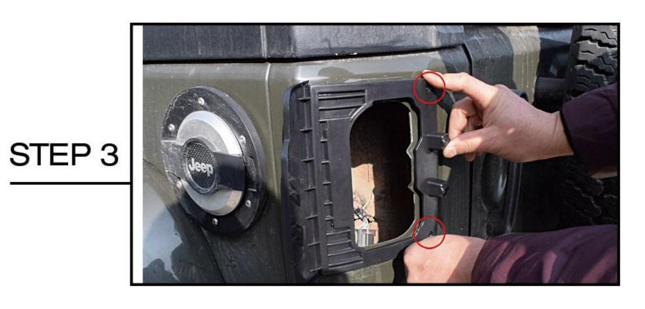
Align the bracket to the position where it needs to be installed. Align the screw holes on the right.
