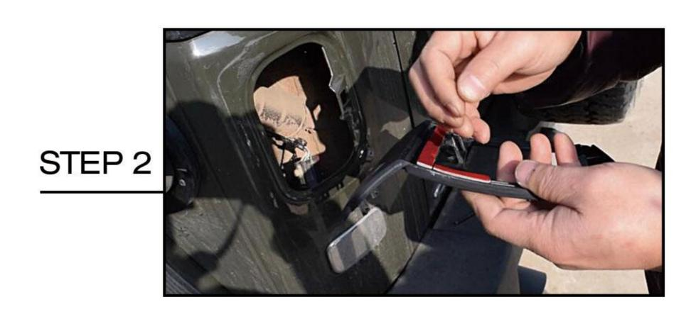
Remove the cover of 3M tape on the bracket.
