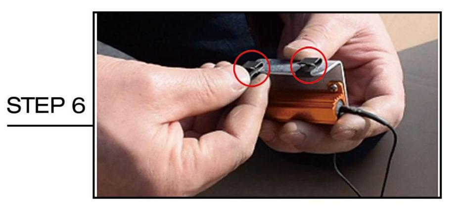
And the black buckle is in the corresponding position of the gasket.
