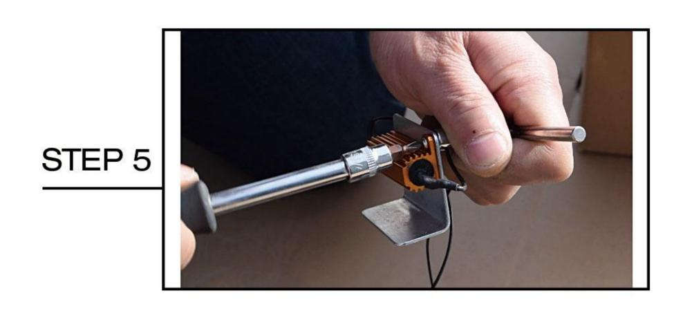
Fix the iron sheet and the resistive decoder with screws.
