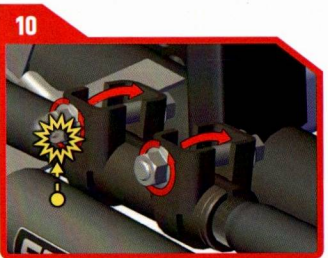
With adjustable track bars, loosen the collar bolts and turn the pinch clamps for proper stabilizer clearance.
