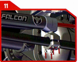
Torque stabilizer tie rod clam shell mount bolts to 15 ft. lbs. Reverify clearance and fitment.
