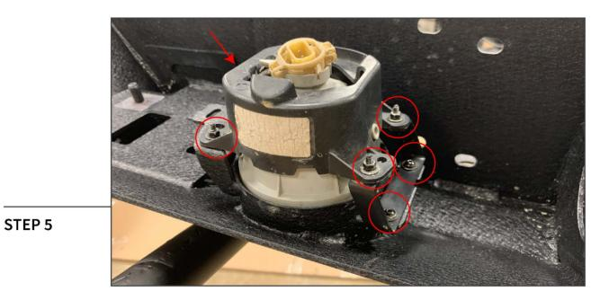
Using 7mm socket and 3mm Allen wrench, install the fog light brackets and factory fog lights to the bumper using the supplied M4 hardware. Each mounting location will use (1) M4 Bolt, (2) M4 Flat Washers, (1) M4 Lock Washer, and (1) M4 Nut.
