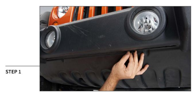
Using a flat head screwdriver, remove the (6) push pins securing the factory splash shield to the vehicle. (4) Across the front and (2) from behind. The splash guard will not be reused.
