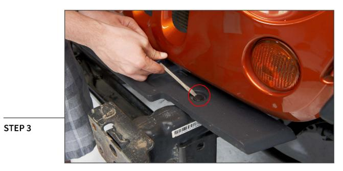
Using a flat head screwdriver, remove the (2) push pins securing the plastic filler panel to the vehicle. The filler panel will not be reused.
