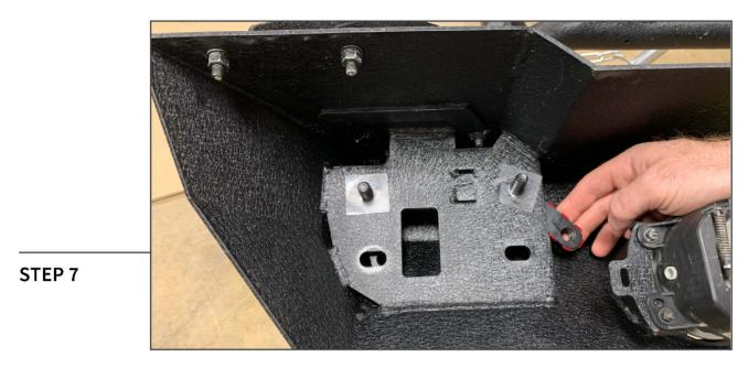
Install the supplied nut plates in front of the bumper mounting pad. Install the plastic retainers over the studs to hold them in place during installation.
