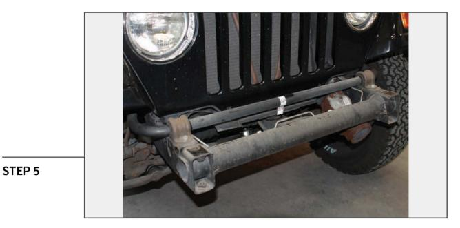
Remove the original bumper from the vehicle. Place the new bumper onto the vehicle frame rails.
