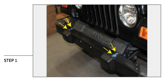
Remove (4) T-55 Torx screws from the top of the bumper.
