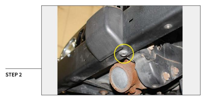
Remove (1) T-55 Torx bolt underneath the bumper on both sides of the vehicle.
