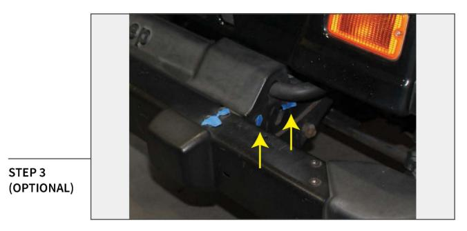
Remove (2) 10mm bolts on each side of the sway bar cover, then remove the cover from the vehicle.
