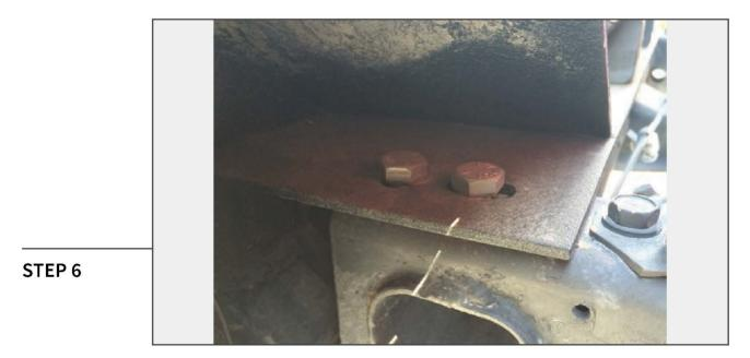
Secure the upper portion of the bumper to the vehicle frame rail using (2) 1/2 x 1.5" bolts, and (2) 1/2" flat washers.
