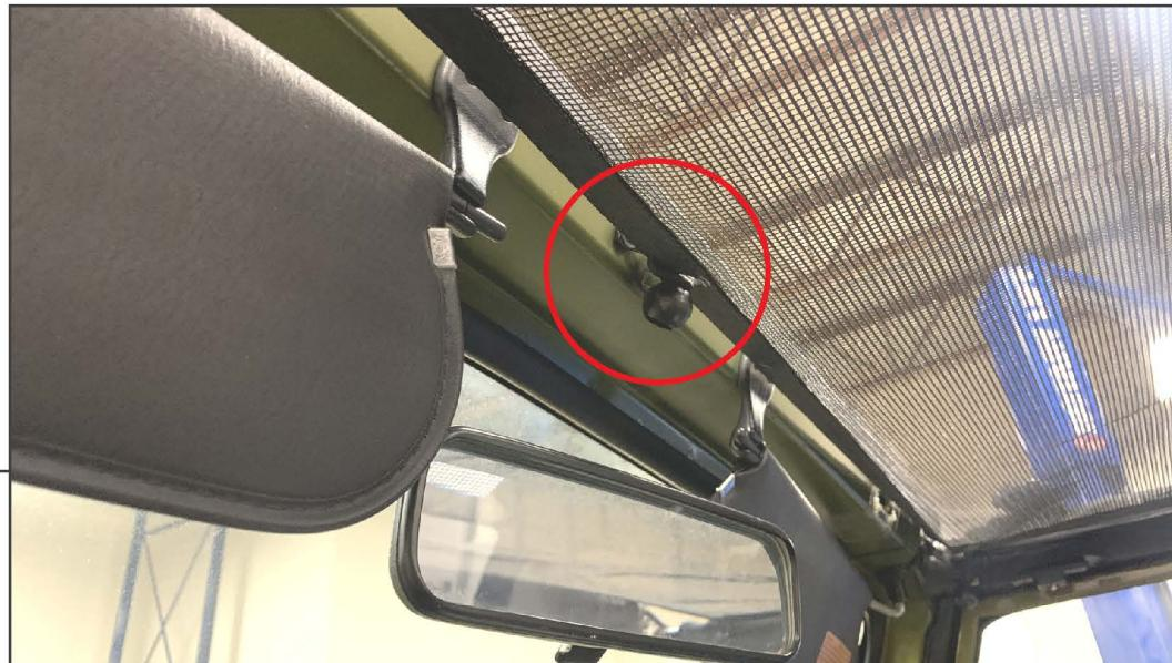
Drape the front of the mesh top over the vehicle center roll bar. Secure the front of the mesh top to the windshield channel using (1) 3" elastic band.
