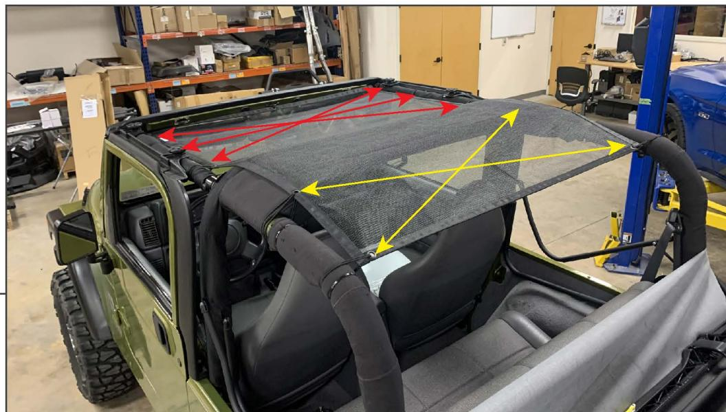
Secure the sides of the mesh top to the roll bar using (6) 5" elastic bands and (4) 8" elastic bands.
