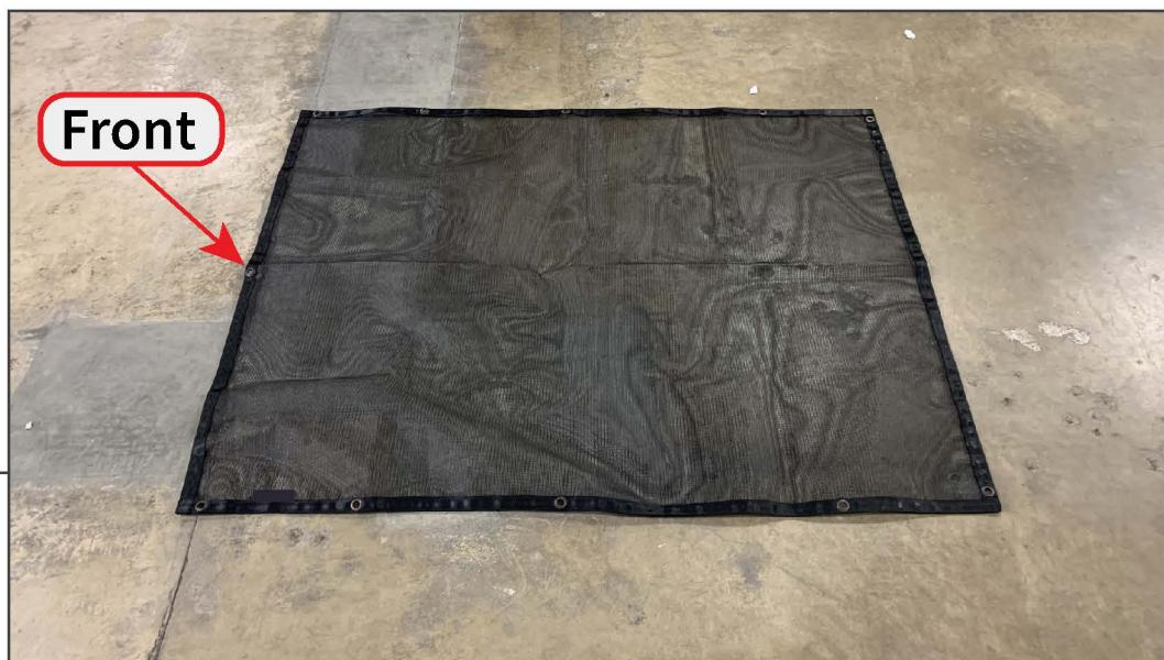
Identify the front of the mesh top by locating the (1) center grommet.
