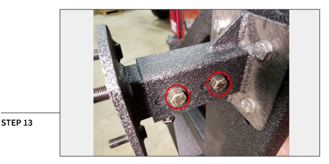
Install the (1) Tire Carrier Mounting Hub to the tire carrier base by using (2) M10 x 120mm bolts, (4) flat washers, and (2) lock nuts. Measure the backspacing of your spare tire by placing a straight edge across the tire. Measure from the mounting hub to the straight edge. Subtract a half inch from the previous measurement, and set the carrier to the new measurement. This insures the tire is against the carrier.
