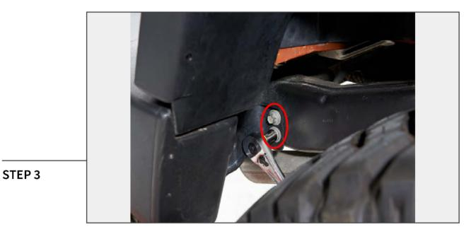
Locate, and remove the (2) 15mm bolts on each side securing the bumper to the frame rail. Remove bumper.
