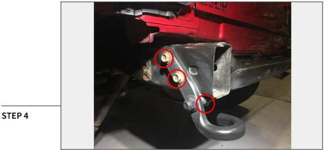
Remove the (3) 15mm bolts securing the tow hook to the driver side frame rail.
