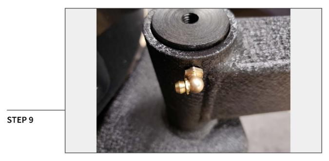
Gently thread the zerk fitting into the tire carrier arm using a 3/8 wrench. **DO NOT OVERTIGHTEN.**
