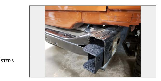
Insert the (2) frame rail brackets into the frame rails, be sure that the holes from the frame rail line up with the bracket holes.
