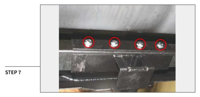
From under the vehicle, secure the center of the bumper using the (4) M12 x 120mm bolts, flat washers, lock washers, and nuts. Torque to 40 ft - lbs.
