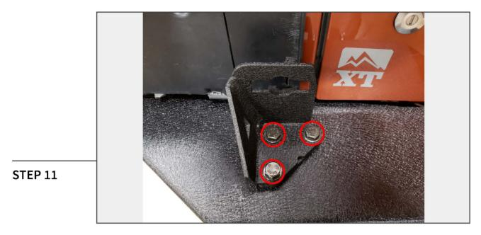
Install the latch bracket to the rear bumper by using the (3) M10 x 40mm bolts, (6) flat washers, and (3) lock nuts. Do not fully tighten, refer to last page for final adjustment.
