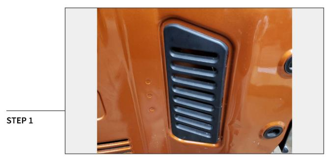
Open the tailgate and remove the vent cover with a trim panel removal tool. Disconnect the brake light wiring harness and reinstall the vent cover.
