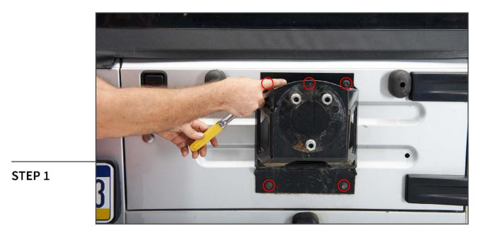
Remove the spare tire from the vehicle. Remove (5) 1/2" bolts securing the tire carrier.
