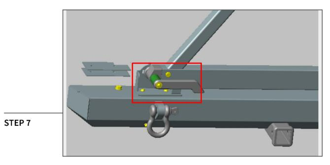
Secure the (1) tire carrier handle bracket to the bumper using (2) M10 x 40mm bolts, (2) M10 lock washers, (4) M10 flat washers, and (2) M10 nuts. Tighten until secure. Use (2) included shims if necessary to add additional height.
