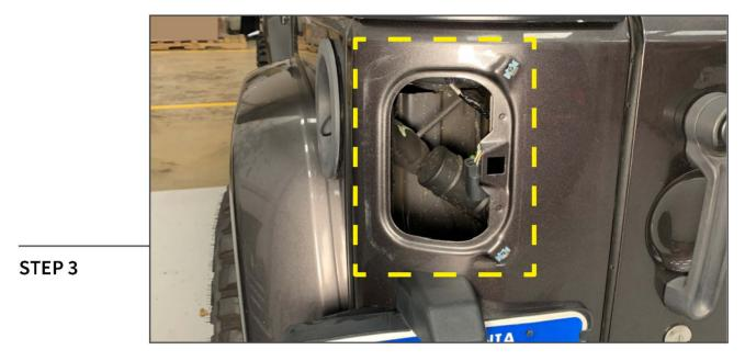
Clean the tail light mounting area of the vehicle using exterior detailer and a microfiber cloth.
