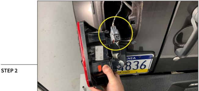
Unplug the (1) electrical connector from the tail light by pressing the plastic tab while separating the harnesses.
