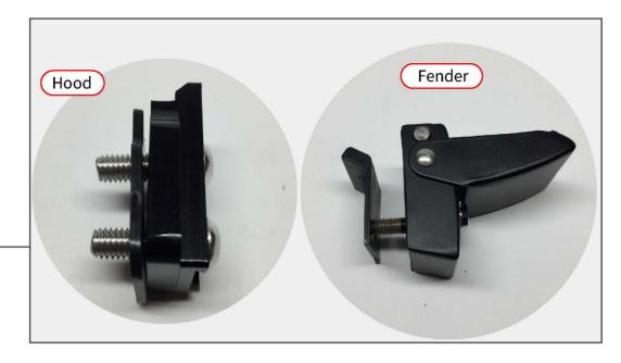
Install the locking latch to the fender using the supplied 13mm lock nut. Install the rubber isolator between the latch and fender. Install the hood latch using the supplied 10mm nuts. Install the rubber isolator between the latch and the hood.
