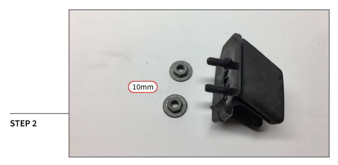
Locate, and remove the (2) 10mm nuts that hold the hood latch to the hood, remove the latch from the vehicle.
