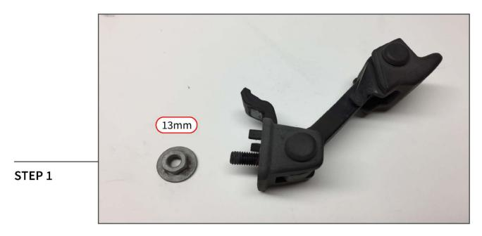
Begin by propping the hood open by unlatching the vehicle hood latch. Locate, and remove the 13mm nut that holds the hood strap to the fender.
