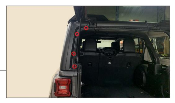
Open the rear window glass, and clean the hardtop area along the gasket using (1) adhesion promoter pad and allow to dry. Adhere (4) wire retainers to the vehicle hard top along the gasket.
