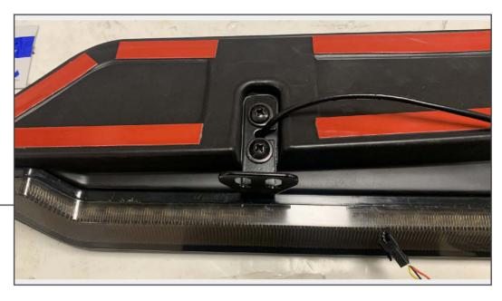
Secure (1) spoiler bracket to the spoiler panel using (2) M5 Phillips bolts, (2) M5 lock washers, and (2) M5 flat washers. Tighten the hardware until the bracket is secure. Ensure the wiring harness is routed into the notch in the bracket.
