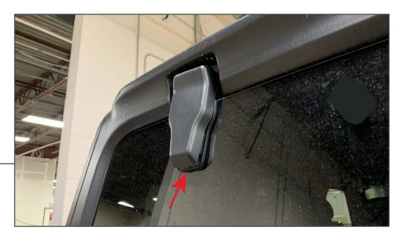
Remove the rear glass hinge cover using a pry tool, and hinge the cover open. Then remove the cover.
