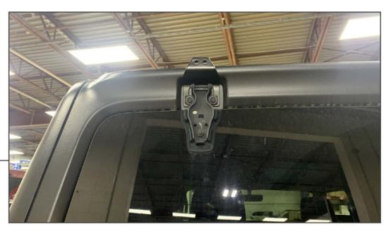
Using a plastic pry tool to gently pull the glass outwards. Insert (1) hinge bracket in between the glass hinge and the vehicle hard top. Secure into place using the (2) original 10mm bolts.
