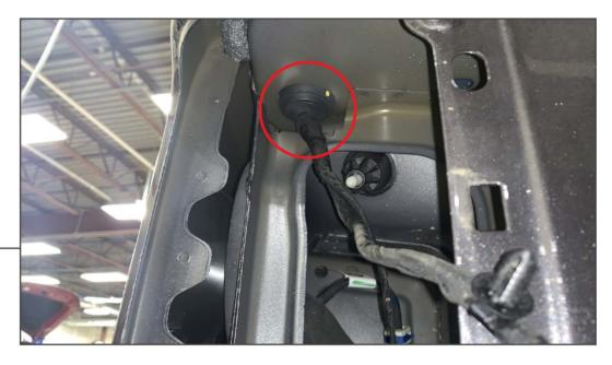
With the tail light removed, locate the wiring harness/grommet routed into the vehicle interior. Carefully cut a slot in the grommet, and route the spoiler panel wiring through towards the vehicle tail light.
