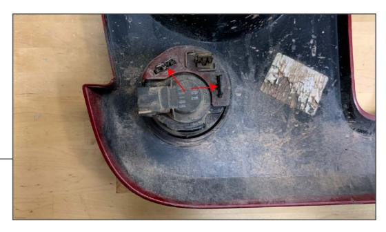
Depress the plastic tabs on the turn signal and push the turn signal out of the factory grille cover. Transfer the removed turn signals into the new grille.
