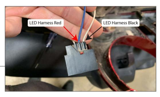
Wiring Instructions: Tap the grille wiring harness into the factory marker light wiring.
