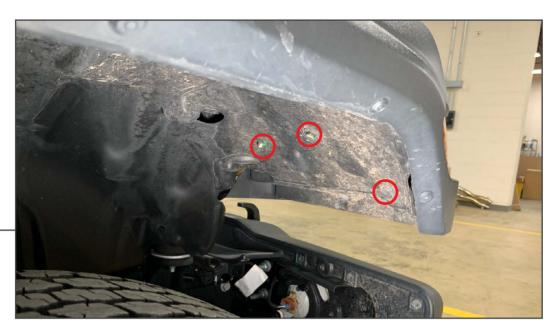
Remove the (2) 8mm bolts and (1) plastic push clip to gain access to the fender mounted running light.
