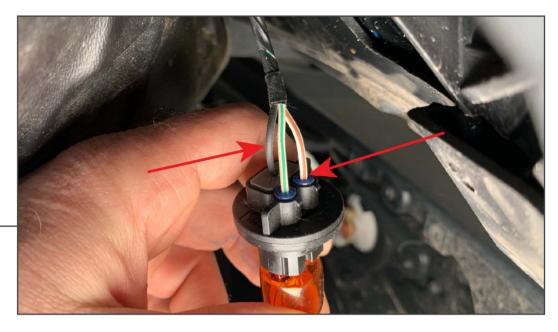
Locate the parking light connector. Splice the grille lighting wiring harness into the parking light following the diagram below. Once wired, re-assemble the fender liner.
