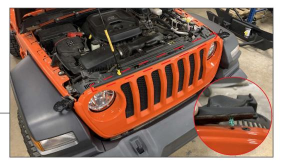
Open the vehicle hood. Remove the upper weatherseal from the grille using a panel removal tool.
