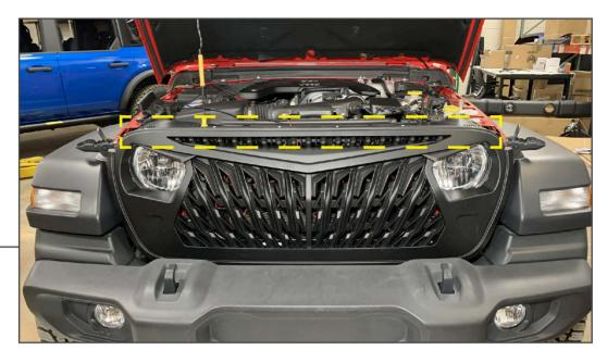
Install the upper weatherseal to the grille assembly by pressing the clips into the pre-drilled holes along the top of the grille. Secure the grille to the vehicle using the (6) original push clips.
