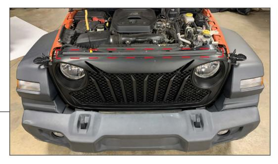
Install the upper weatherseal to the grille assembly by pressing the clips into the pre-drilled holes along the top of the grille.
