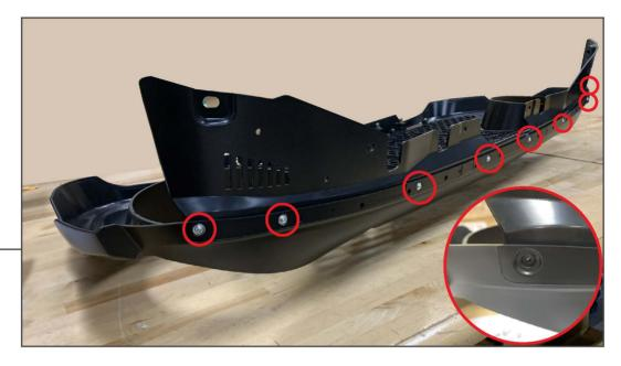
Align the upper mounting bracket under the upper grille lip. Secure the mounting bracket to the grille using (8) M4 bolts, (8) M4 flat washers, and (8) M4 flange nuts. Ensure to only install the hardware in the holes with the cutout for the flat washer.
