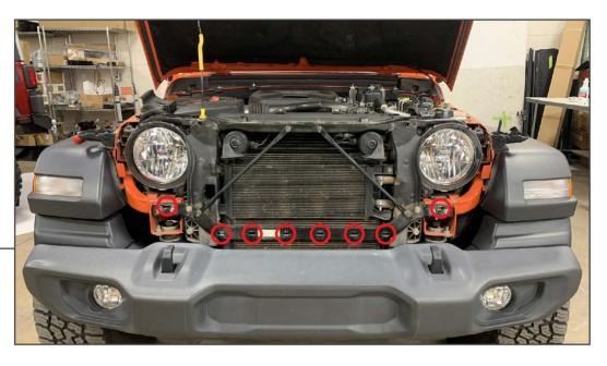
Firmly pull the bottom of the grille away from the vehicle to dislodge the (8) grille vampire clips.
