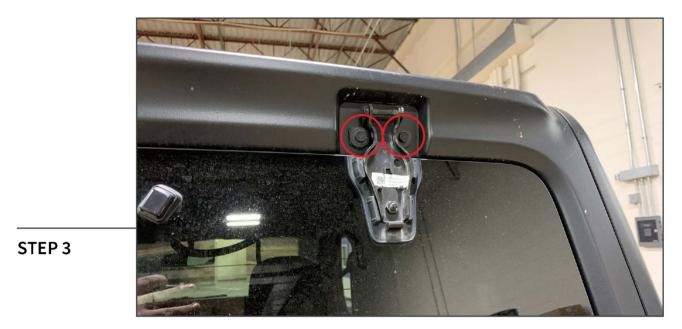
Remove (2) 10mm bolts from the hard top hinge.
