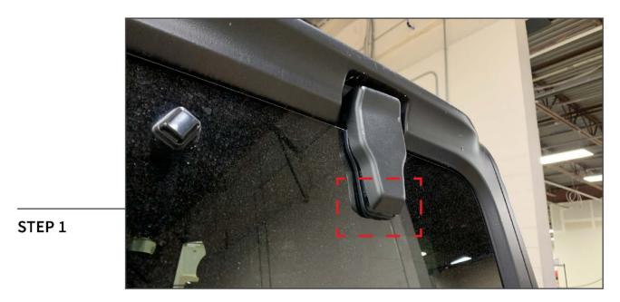
Using a panel removal tool, pry the bottom of the rear glass hinge cover to release the retaining clips.
