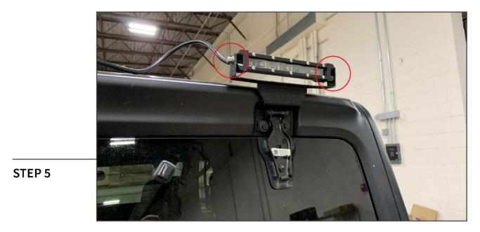
Install the LED to the mounting bracket using (2) M6x1.00 x 15mm Allen bolts, (2) M6 lock washers, and (2) M6 flat washers.
