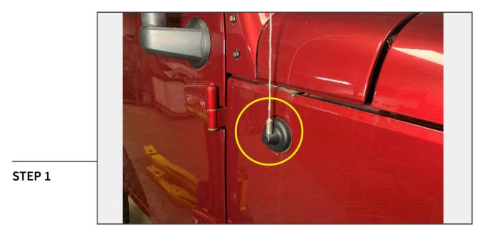
Clean vehicle. Remove vehicle antenna using an adjustable wrench.
