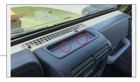
Remove the dashboard rubber mat, and remove the (2) screws from the vehicle dashboard.
