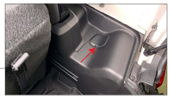
Begin by opening the tailgate to access tail light trim cover. Using a soft pry tool, remove the cover from the vehicle.
