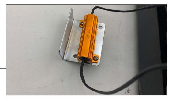
Using a Phillips head screwdriver and a pair of pliers, install the resistors to the resistor mounting bracket. Each resistor will require (2) machine screws and (2) lock nuts.
