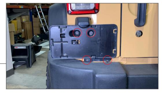
Remove vehicle license plate. Remove (4) 7mm screws from the license plate mount.
