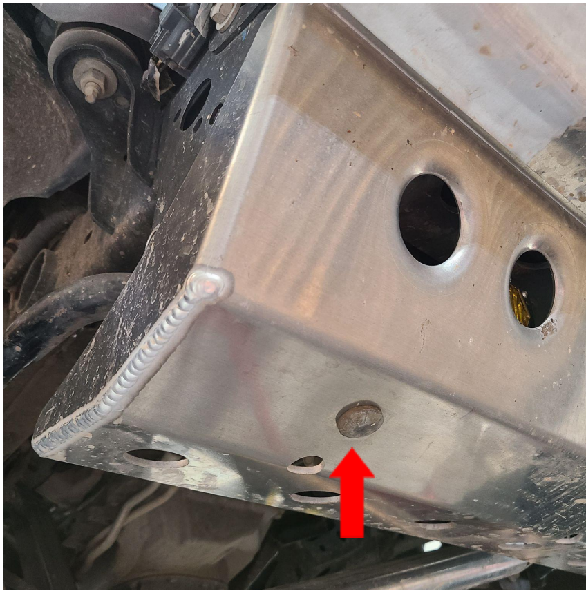
Figure 12: Red arrow calls out final mounting location for lower skid using \frac{1}{2} " carriage bolts
