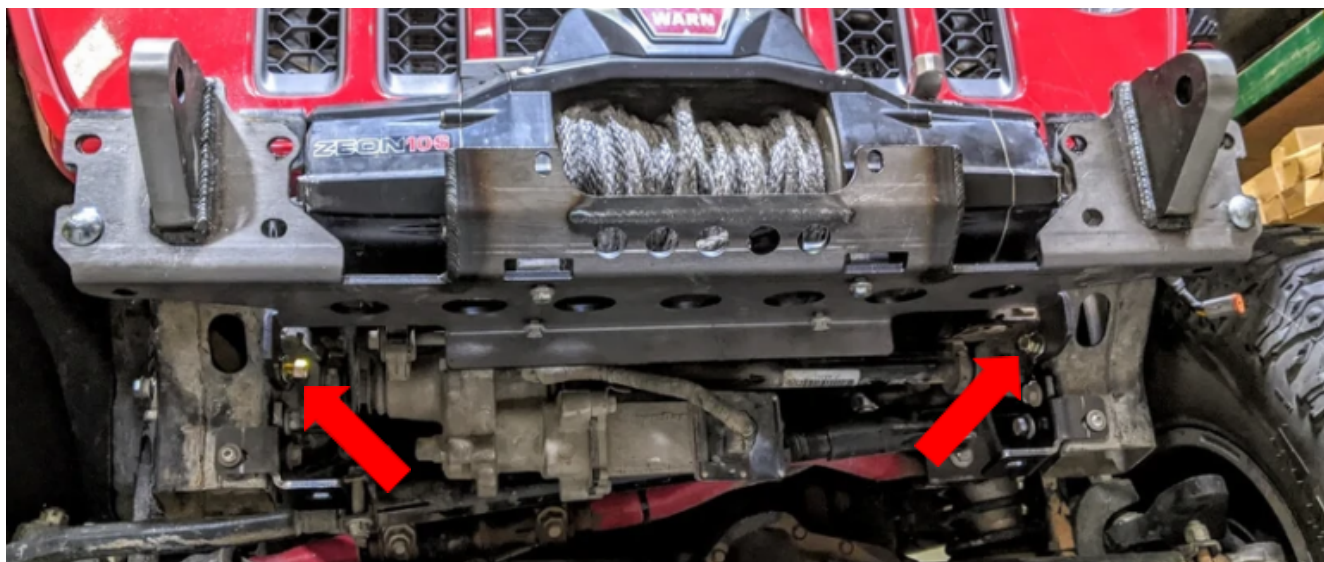
Figure 4a: Red arrows call out the mounting locations to fasten the winch tray to the sides of the frame rails.
