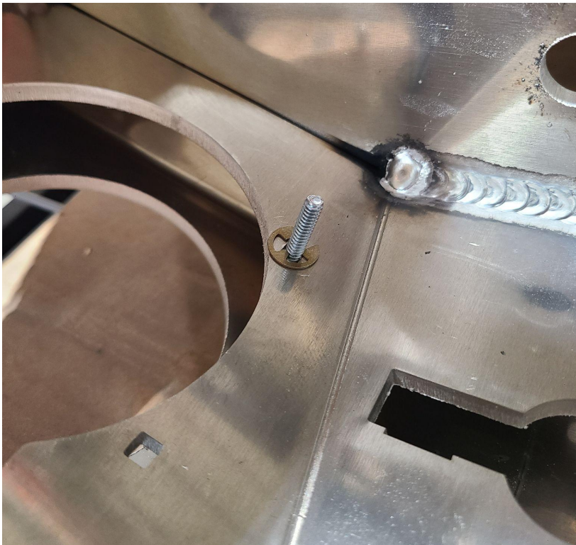
Figure 17: Install 10-24 carriage bolts with retaining rings before installing factory fog lights
