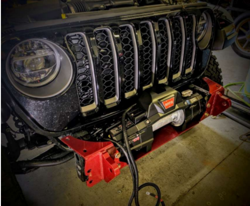
Figure 5: Winch installed into winch tray
