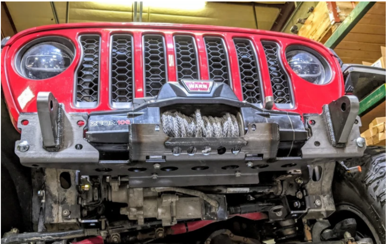
Figure 3: Steel Winch Tray Mounted
