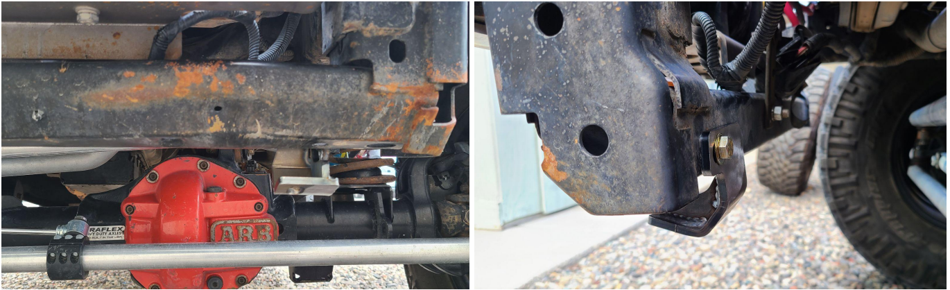
Figure 8: Lower Front Skid Plate Driver Side Bracket Installed
