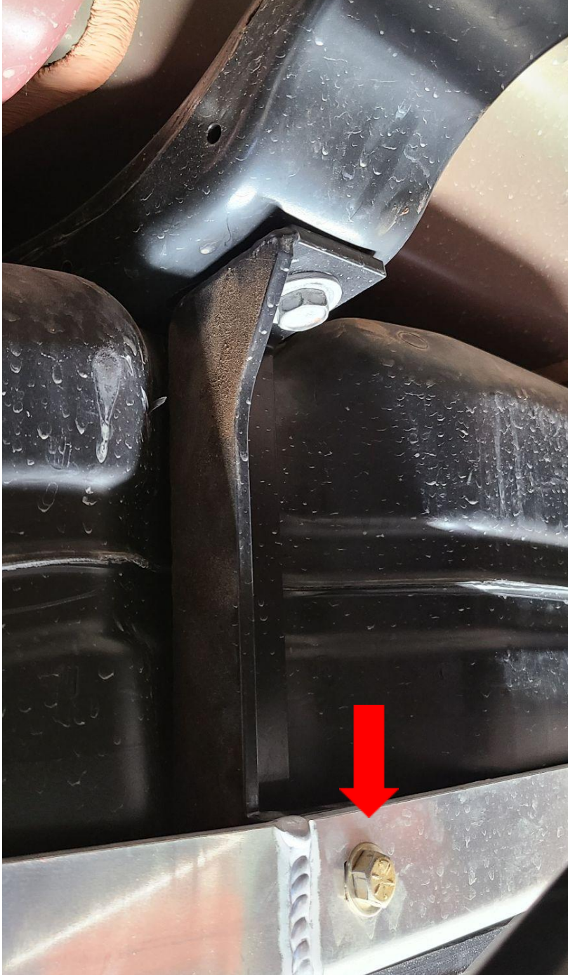
Figure 12: Fuel tank mount to crossmember I (Figure 3 Item #5) will utilize a provided \frac{3}{8} "-16x1.25" carriage bolt, washer, and nut (Figure 2 Items #4, 5, 6) rather than the hex head bolt pictured here.
