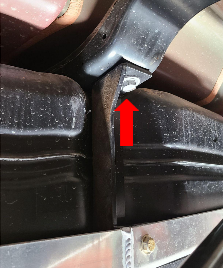
Figure 6: Inside mounting location of rear fuel tank support I (Figure 3 Item #5) will utilize factory hardware.
