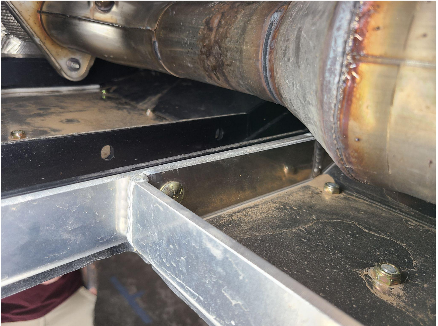
Figure 22: This mounting location (exhaust, transfer case, and main crossmember) will utilize the 1 provided \frac{3}{8} "-16x1.5 hex head bolt, washers, and nut (Figure 2 Items #12, 5, 6)
