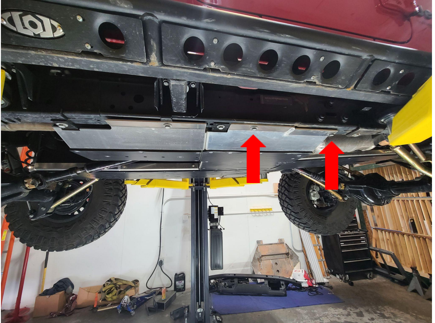
Figure 17: Passenger frame rail mounting locations will use factory hardware. Please note that the forward most mounting location called out above may require the use of the provided nut stick Q (Figure 3 Item #19). If your Jeep's frame already has a factory threaded insert, this nut stick will not be used.
