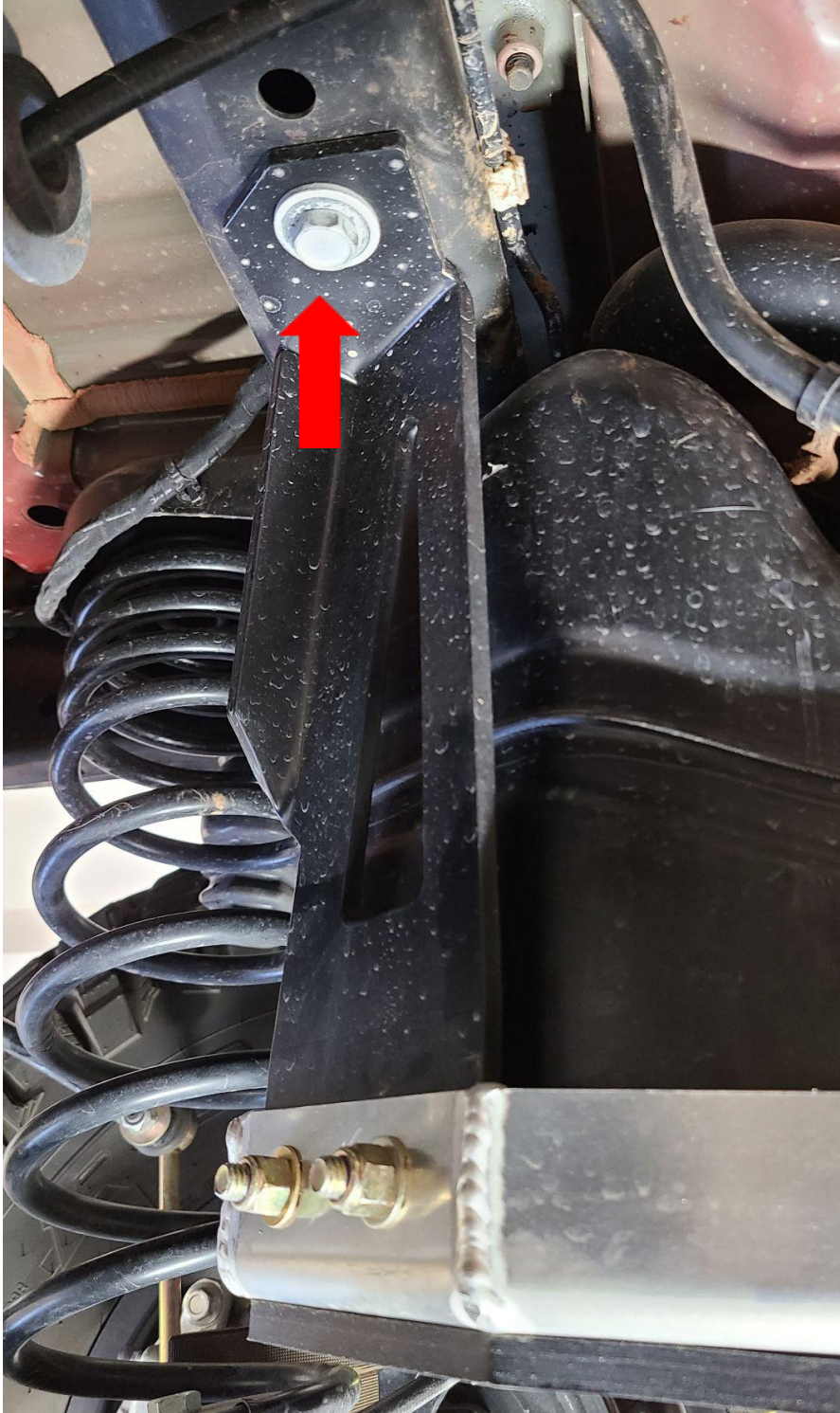
Figure 10-JL: Rear fuel tank support bracket L (Figure 3 Item #7) mounting location on the frame will utilize factory hardware. See slight differences in install for JT version of this bracket below:
