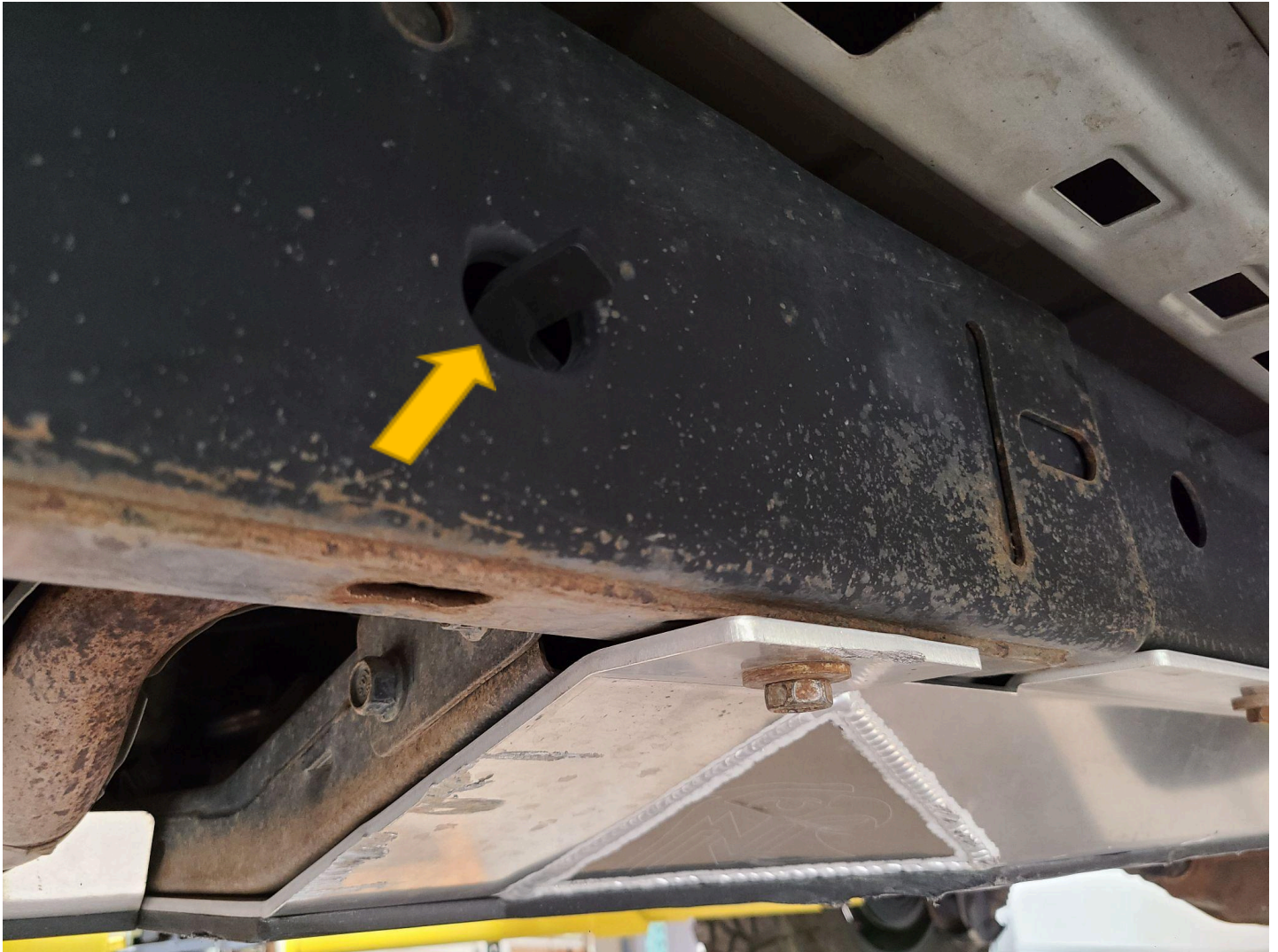
Figure 6. Installation orientation of nut stick "O"
