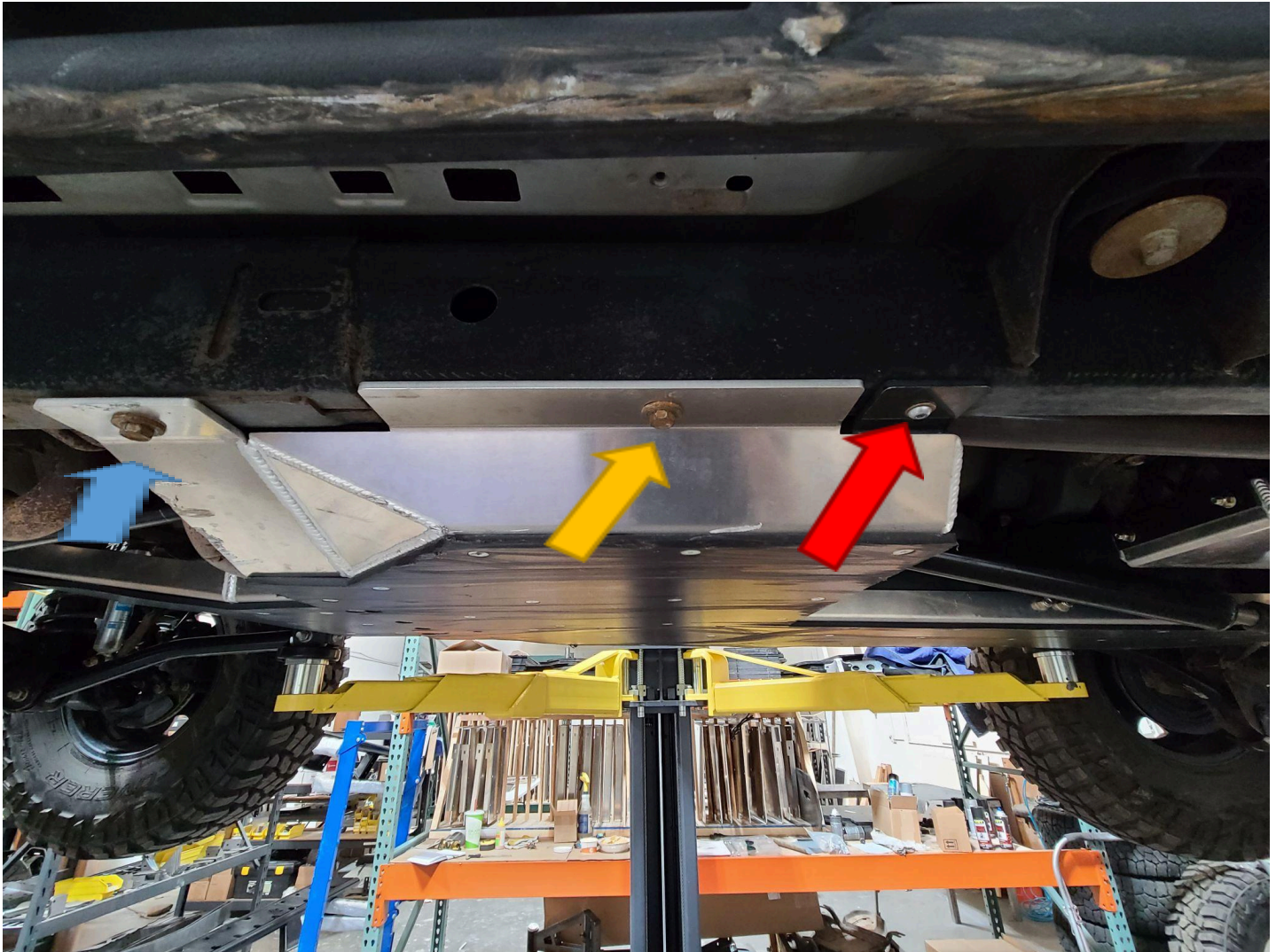
Figure 5. Driver side frame rail transfer case skid mounting locations
