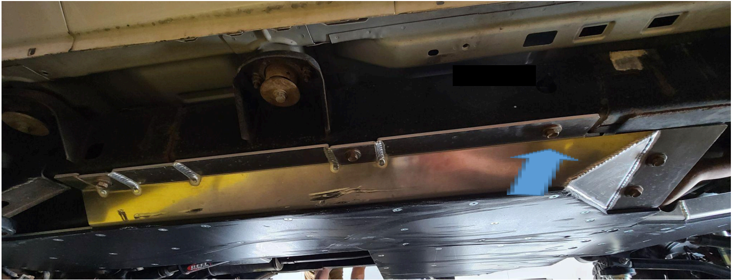
Figure 7. Passenger side skid plate mounting locations
