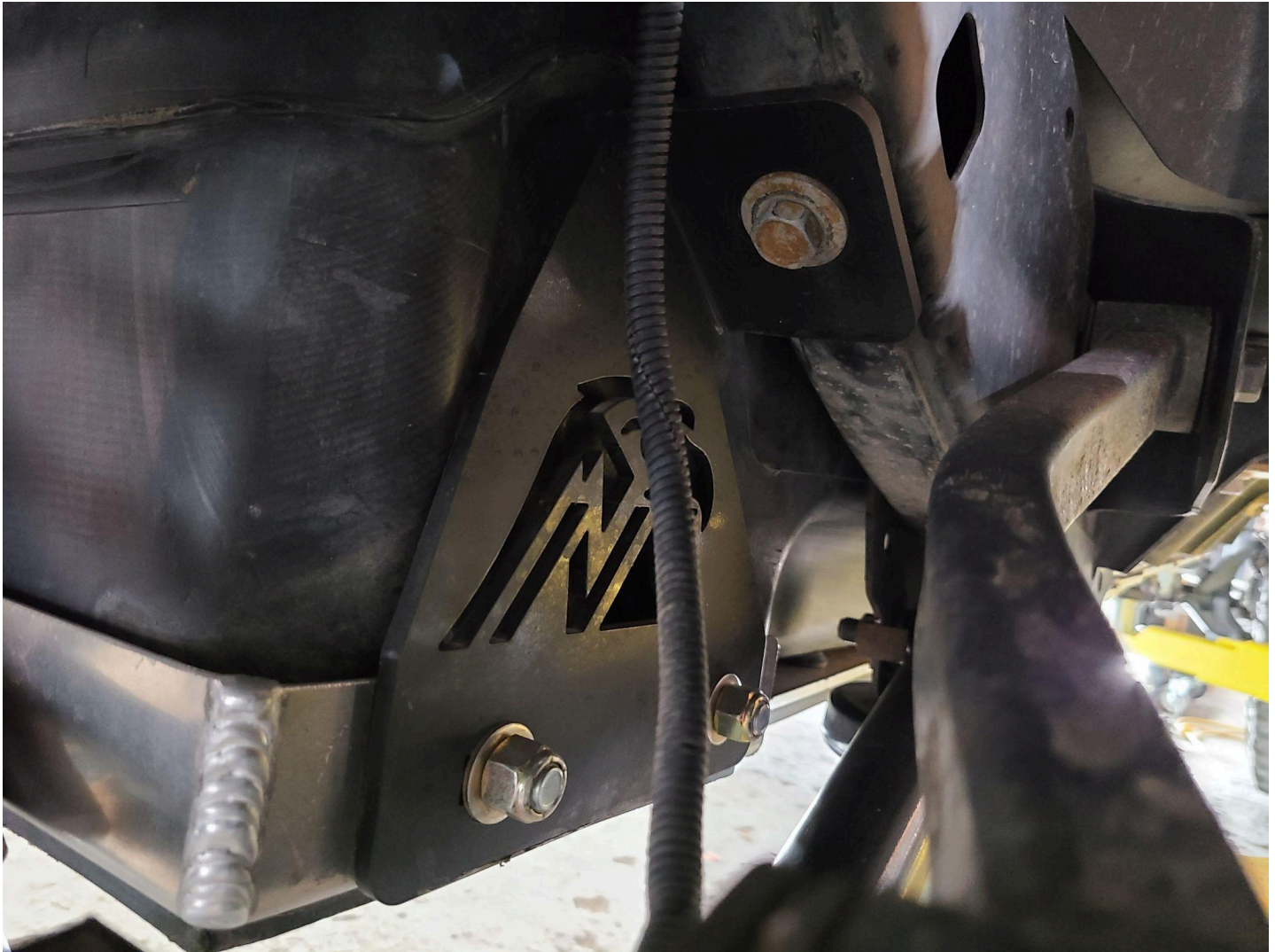
Figure 11. Bracket N Installation
