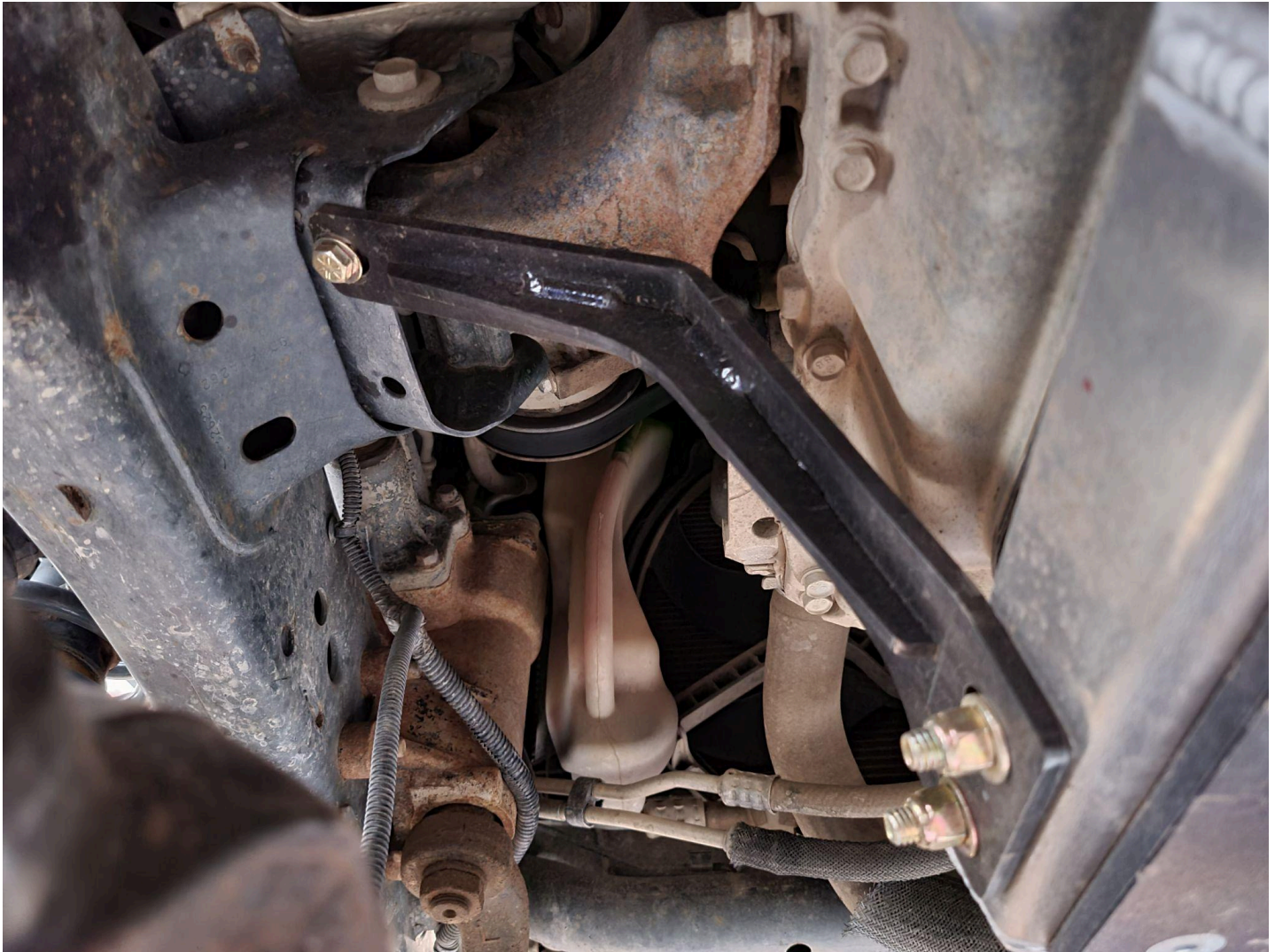
Figure 13. Driver side bracket D installation
