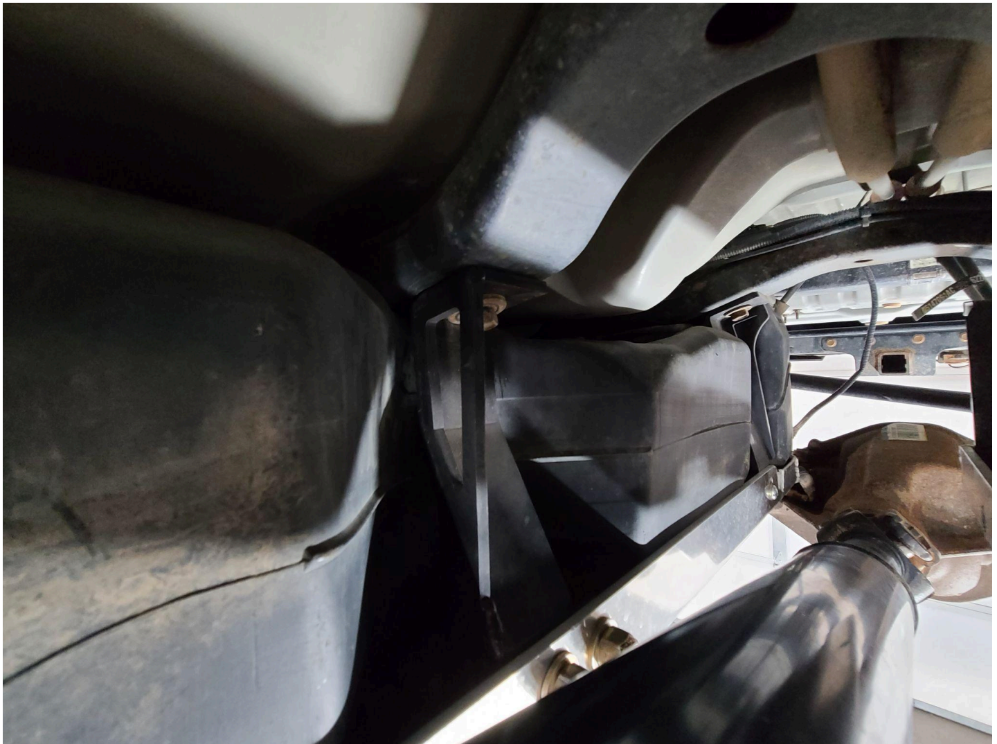
Figure 10. Bracket H Installation. Note that these bolts should be installed opposite of the photo shown, with the nuts on the inside of the fuel tank skid. This will allow for more clearance with your driveshaft.
