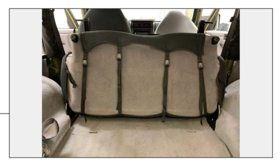
Install the cover over the seat bottom. Push the straps through the seat back and loop them under the seat. Reconnect the straps under the seat. It is helpful to fold the seat up during this process.
