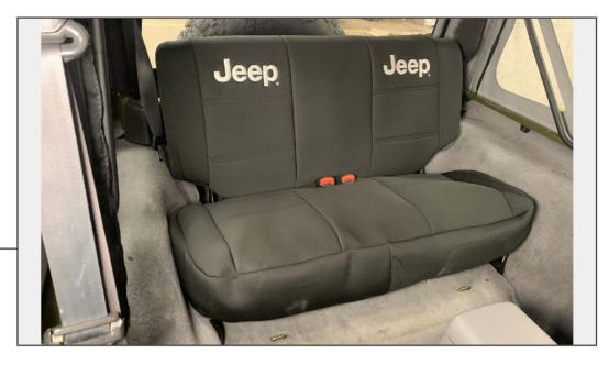
Fold down and latch the rear seat. Then, push the rear seat belt buckles through the seat bottom to complete the seat cover installation.
