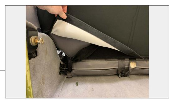
Install the seat back cover over the top of the seat. Pull the cover down the seat. Push the soft portion of the seat cover through the seat towards the back of the vehicle. Pull the soft portion up the back of the seat and attach it to the back side of the seat cover.
