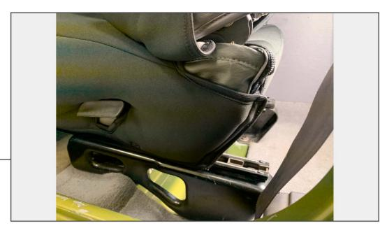
Place the bottom cover over the seat. Push the straps through the back of the seat and loop them under the seat bottom. Position the seat lever through the hole in the cover. Wrap the hook and loop portion of the bottom cover around bottom of the seat and attach.
