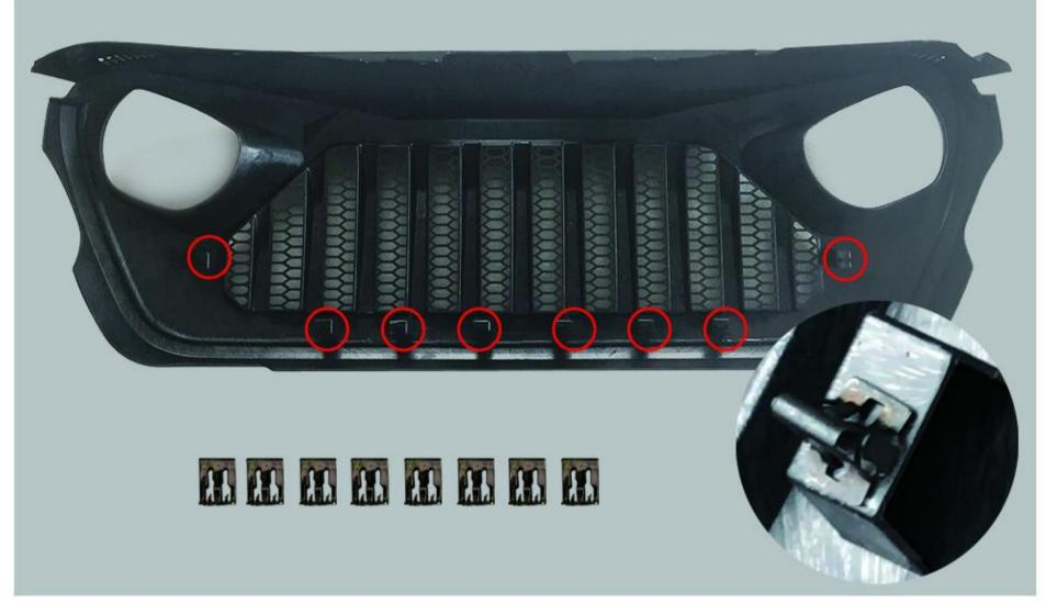
Step 2: Install the retaining clips(8) in the appropriate position on the back of the grille.
