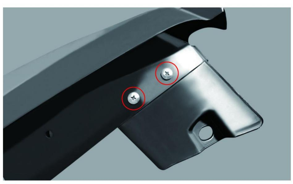
Step 3: Fix the bracket with screws.
