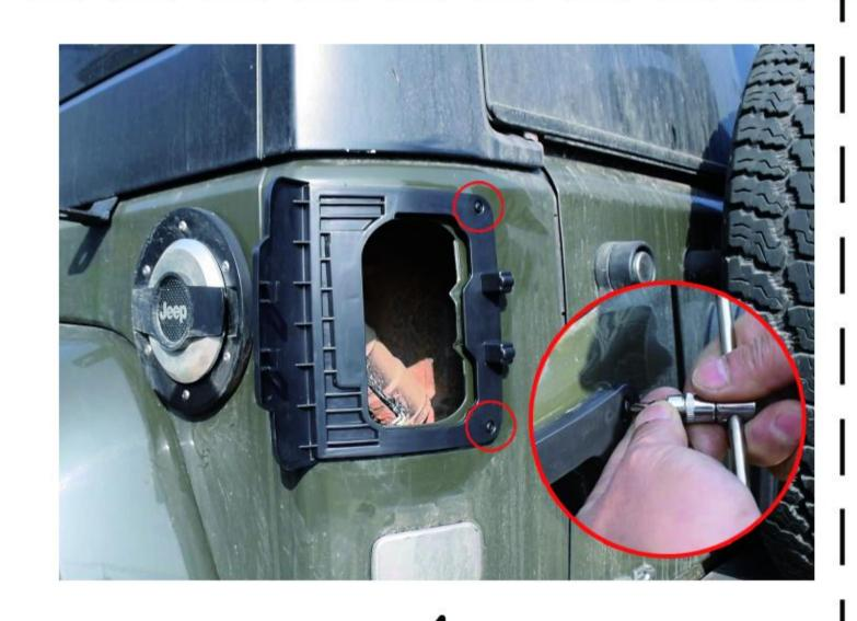
Fix the bracket with the 2 mounts in the packages. Make sure the stand does not shake.
