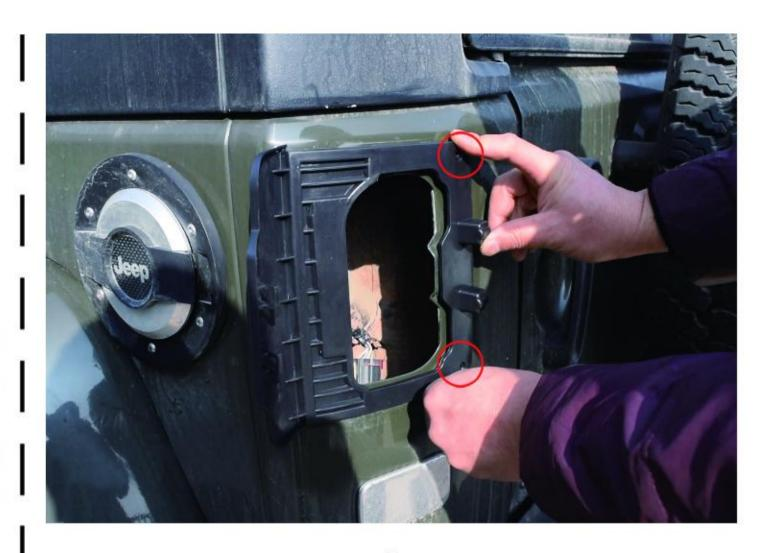
Remove the cover of 3M tape on the bracket. | Align the bracket to the position where it needs to be installed. Align the screw holes on the right.
