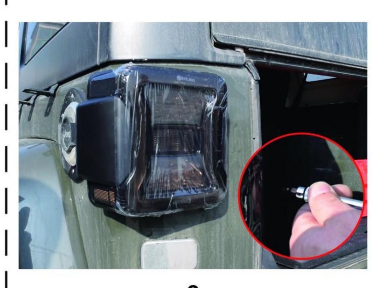
Fix the taillights assembly to the brackets, and fix with screws to complete the overall installation.
