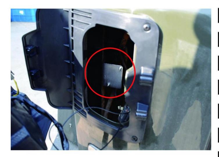
Fix the assembled gasket in the corresponding position of the car.
