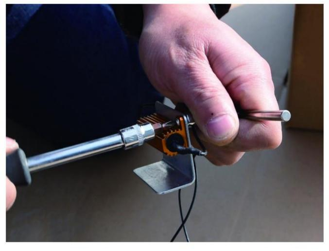
Fix the iron sheet and the resistive decoder with screws.
