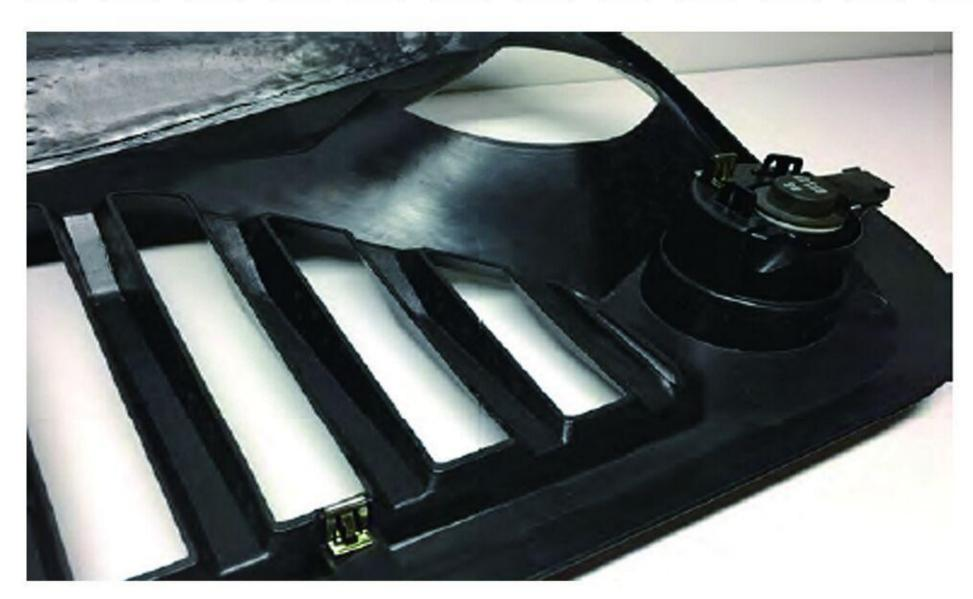
Step 3: Press on the (6) supplied retaining clips. Using the factory grille as a reference, apply the supplied weather stripping across the top of the grille.
