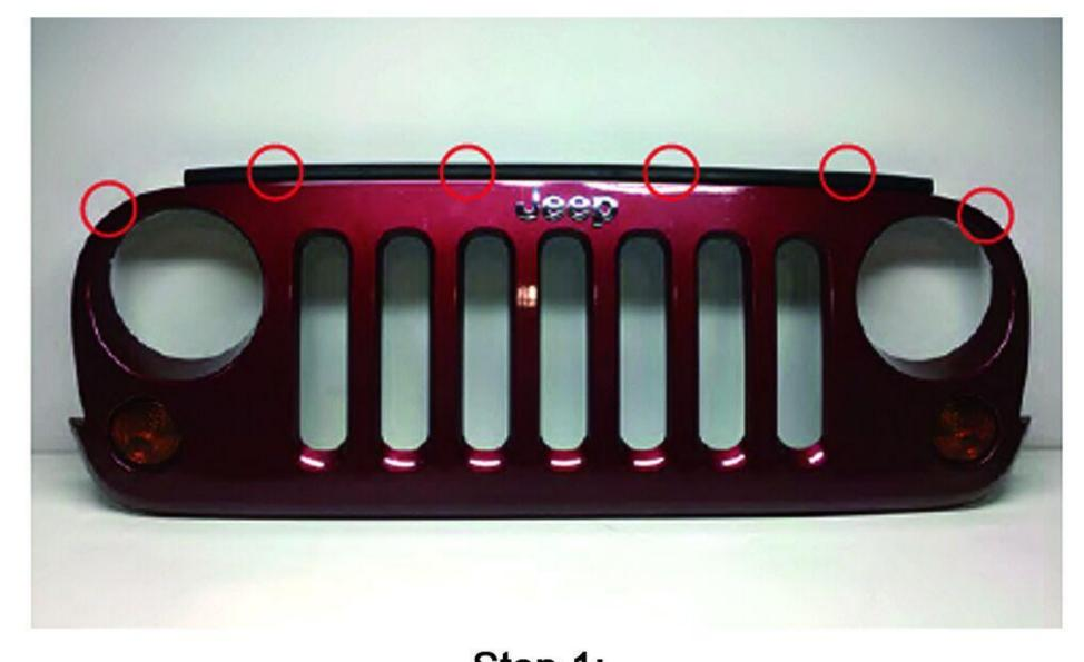
Step 1: Using a panel removal tool, remove the (6) push clipsholding the grille cover to the vehicle. Unplug the turnsignals and pull the grille cover from the vehicle.
