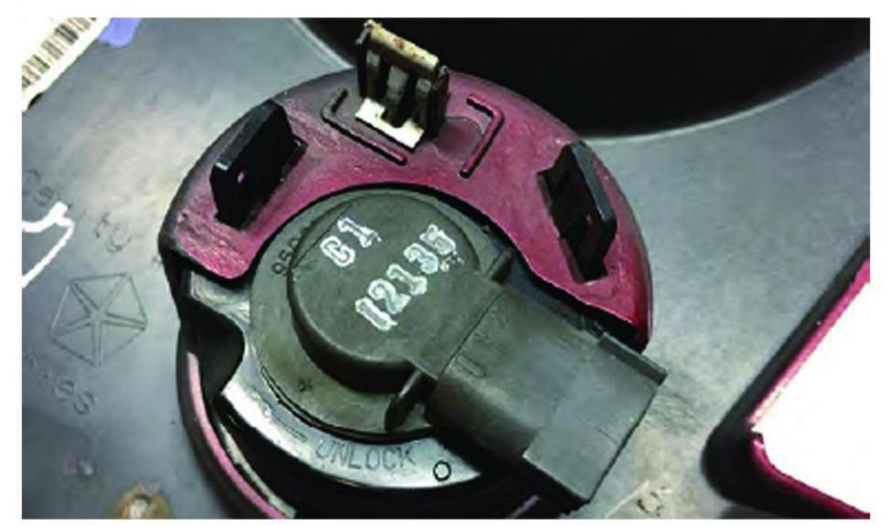
Step 2: Remove the factory turn signals by unclipping them from the factory grille. Transfer them to the new grille.
