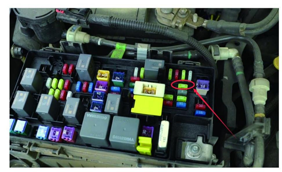
Step 4: Connect the red and black wire of the light bar to ACC and negative of battery.
