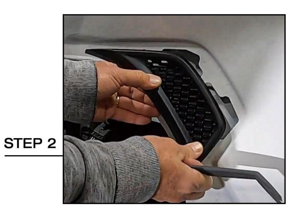
Use tool to remove the original side fender vent from the vehicle.
