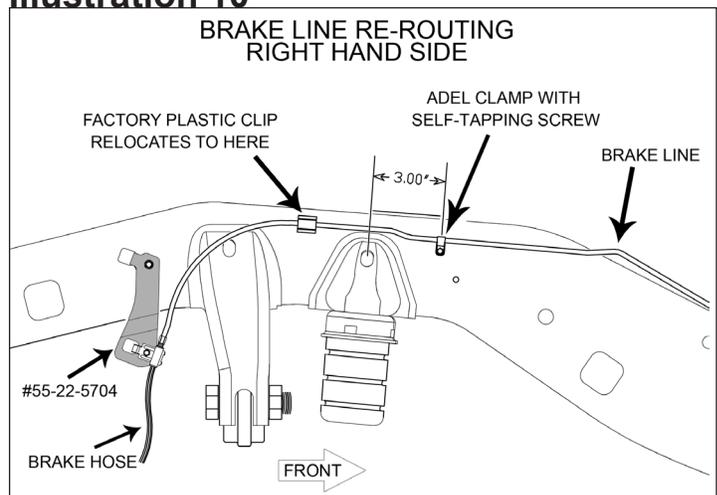
sure 1-3/8" down from the top of the frame rail and 3" forward of the compression travel dampener mount's centerline. At this point, drill a 7/32" pilot hole for the self-tapping screw.
