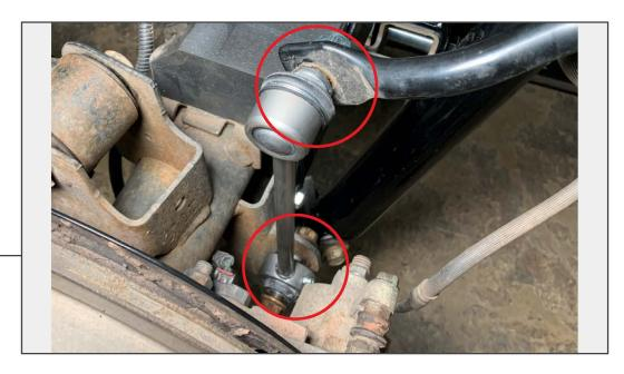
Install the new sway bar links into the vehicle, use the provided lock nut to secure the sway bar link to the sway bar, then use the original hardware for fastening to the axle.
