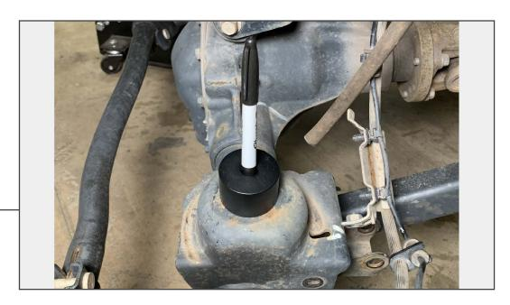
Using a permanent marker and the provided bump stop, make a mark onto the center of the spring perch for drilling. Drill this hole using a 3/8" drill bit.
