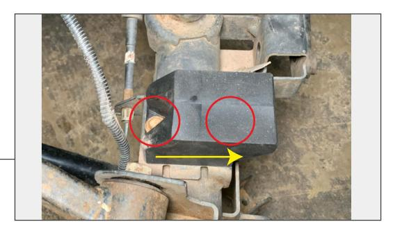
Install the bump stop to the rear axle using (2) 5/16 bolts, nuts, and washers. Make note of the direction of the bump stop.
