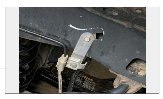
Install the brake line extension to the brake line bracket. Bolt the extension to the frame using original hardware. Gently massage the brake line to ensure the brake line is not touching the vehicle.
