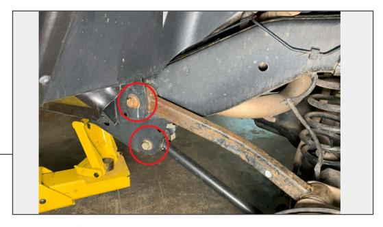
Loosen, but do not remove, the (2) 21mm control arm bolts from the frame.
