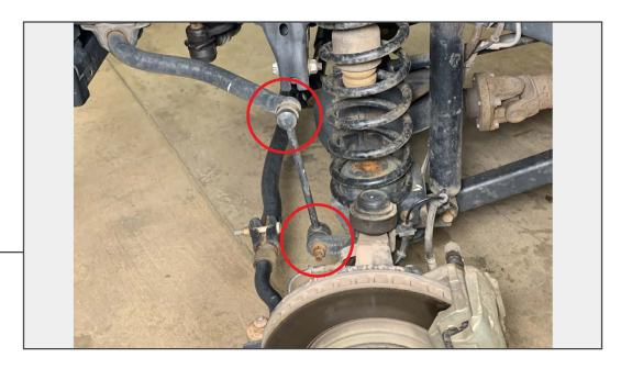
Remove the sway bar links from the vehicle. Remove the top 19mm nut, then the 18mm bolt from the bottom of the sway bar links.
