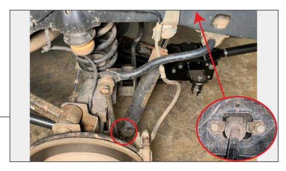
With the axle supported, remove (1) 18mm nut and bolt from the lower shock mount, then remove (2) 16mm bolts securing the upper mount to the frame. Remove the shock from the vehicle. Hardware will be reused.
