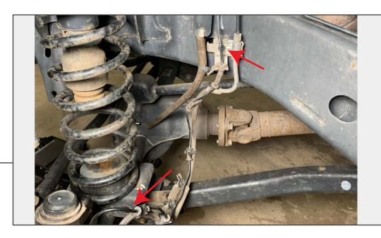
Remove the (2) 10mm bolts to release the brake line brackets from the vehicle. This will allow additional slack when lowering the axle.
