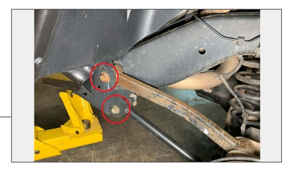
Reinstall the vehicle wheels to the vehicle. Lower the vehicle to the ground, and tighten the control arm bolts attached to the frame to 125 ft-lbs.
