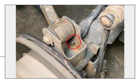
Remove the wiring harness from the control arm mount using a panel removal tool.
