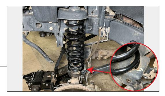
Install the new front spring (taller spring) into the vehicle. Be sure to align the bottom of the spring with the cutout in the axle.
