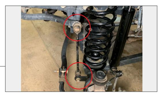
Install the sway bar links previously on the rear to the front sway bar using original hardware.
