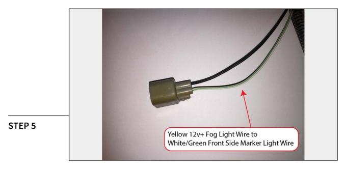
Plug the fog light into the vehicle fog light wiring harness. Splice the additional (1) Yellow wire lead to the vehicle parking light wiring in the fender flare (White/Green 12v+ wire) using the provided Scotchlok connector.
