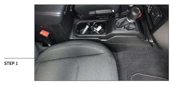
Clean the center console area of the vehicle using isopropyl alcohol and a microfiber cloth, and allow the panel to dry. Test fit the storage tray to the vehicle prior to removing the tape backing.
