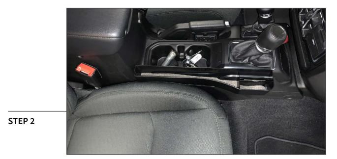
Peel the red tape backing from the storage tray, then adhere the tray to the vehicle. Firmly apply pressure to ensure proper adhesion.
