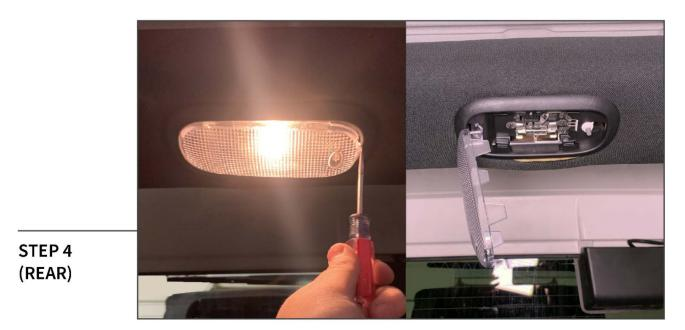
Gently remove the dome light cover using a pry tool/flathead screwdriver in the visible cutout. The cover will hinge downwards.
