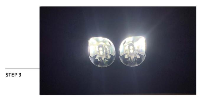
Install the new LED light bulbs into the dome light and test functionality. Once tested, reinstall the plastic dome light cover to the vehicle by pressing the cover into place until an audible click is heard.
