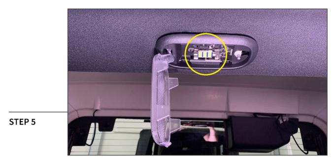
Remove the (1) light bulb from the rear dome light. Install the new LED light bulb into the dome light and test functionality.
