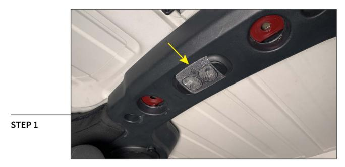
Gently remove the dome light cover using a pry tool/flathead screwdriver.
