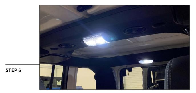
Once tested, reinstall the plastic dome light cover to the vehicle by pressing the cover into place until an audible click is heard.
