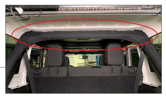
Unzip the upper rear roll bar to reveal the steel roll bar.
