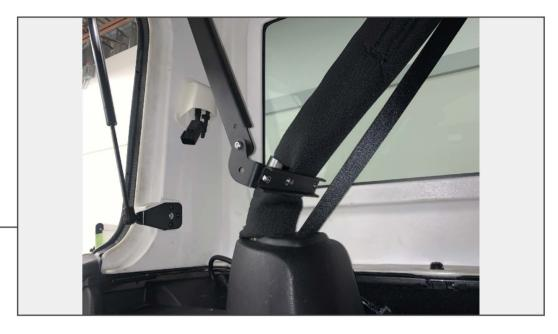
Loosely install each assembled bracket to the lower roll bar using (2)  $M6x1.00 \times 45mm$  Allen bolts and (2) M6 lock nuts.
