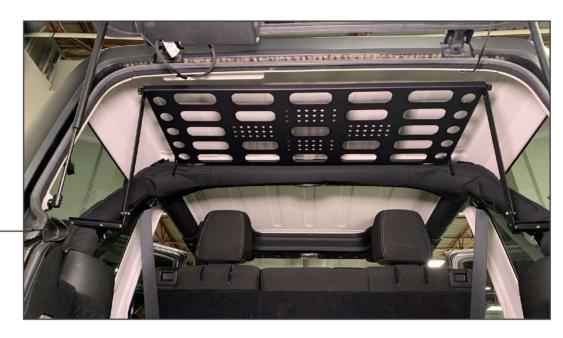
To fold the molle panel parallel with the vehicle top, remove the (2) threaded knobs, and lift the molle panel upwards, and resecure to the brackets using the (2) threaded knobs.
