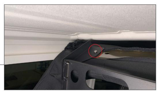
Mount the overhead molle panel with the mounting brackets to the vehicle roll bar using (1) M8x1.25 x 25mm Allen bolt on each side, tighten until secure.
