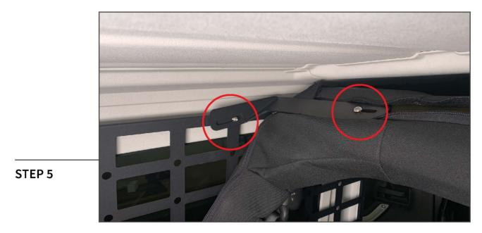
Align the (1) 'L' bracket to the roll bar and loosely secure using (1) M8 x 25mm Allen bolt. Loosely secure the molle panel to the 'L' bracket using (1) M6 x 15mm Allen bolt and (1) M6 flange nut. Adjust the bracket and molle panel as necessary for best fit. Tighten all hardware.
