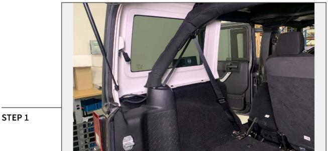
Remove (3) T-40 Torx bolts from the side of the hard top.
