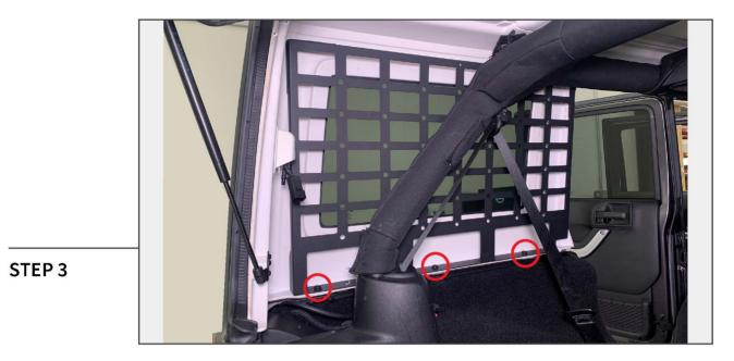
Place the molle panel to the vehicle hard top, and loosely secure the panel to the hard top using the original (3) T-40 Torx bolts.
