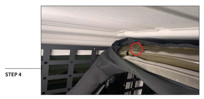
Un-zip the upper roll bar cover to reveal the metal roll bar. Locate the (1) threaded insert in the roll bar.
