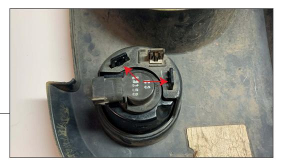
Using a flathead screwdriver, push in the (2) locking tabs holding the turn signal housing into the grille. Once unclipped, push the fog light housing through the front of the grille. Repeat procedure to the opposite side of the grille.
