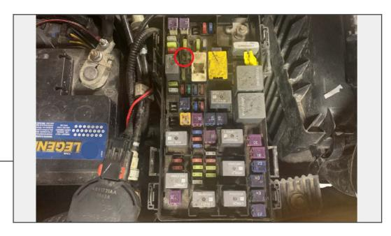
Insert the (1) fuse tap into the fuse box at the indicated location [M9]. If fuse spot is currently used, remove the fuse and replace a fuse in the fuse tap prior to installation. Route the fuse tap out of the fuse box and crimp to the grille DRL wiring harness.
