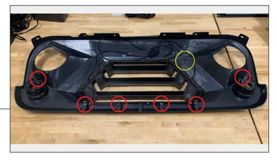
Place (6) vampire clips onto the back of the grille. Neatly route the DRL lighting harness to a suitable location and adhere the module.
