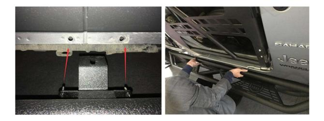
**Step 3**:Then tighten the bolts on the three parts. You may have to lie under the chassis to screw the bolts.
