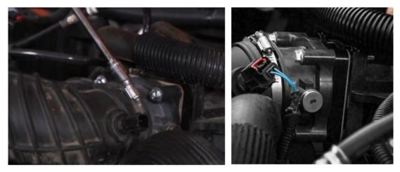
Notes: Don't over tighten the bolts. If the bolts are over tightened the throttle body can be damaged.
