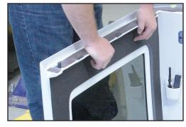
3.) Peel paper backing slowly and press fit piece as you pull backing off.
