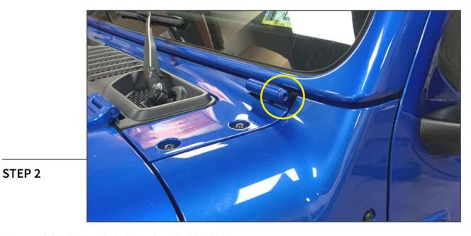
Remove (1) T-50 Torx bolt from the windshield hinge.
