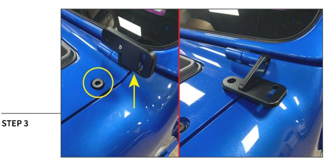
Install the cowl light mount to the winshield hinge using the provided (1) 6mm Allen bolt. Place (1) provided spacer inside the bolt hole on the cowl. Fold the light mount to rest on the spacer.
