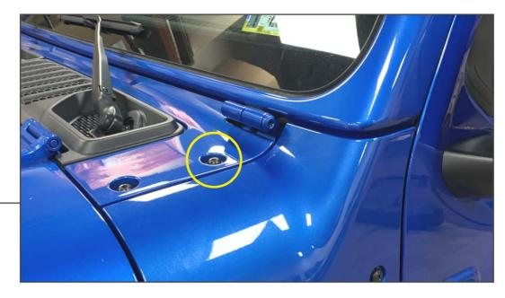
Remove (1) T-40 Torx bolt from the vehicle cowl.
