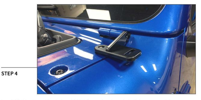
Install (1) M6 x 45mm Allen bolt and (1) M6 flat washer through the light mount and the spacer. Tighten the hardware evenly to secure the light mount to the vehicle.
